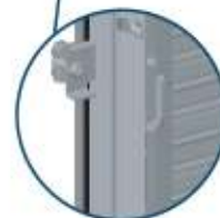
Detail C Manual opening mechanism
